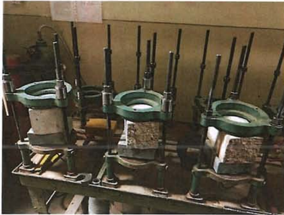
Figure 4.1. Equipment and prepared samples for water absorbtion test. Inside of the sample V3 after testing
