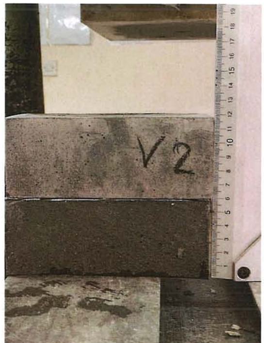
Figure 4.2. Measurement of water penetration depth on samples V1 and V2
