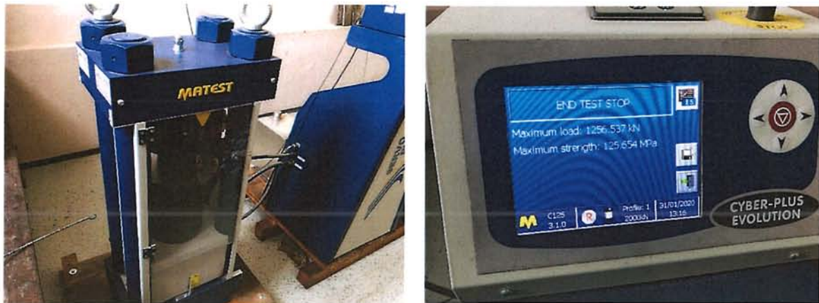
Figure 2.1. Equipment for compressive strength test Matest
