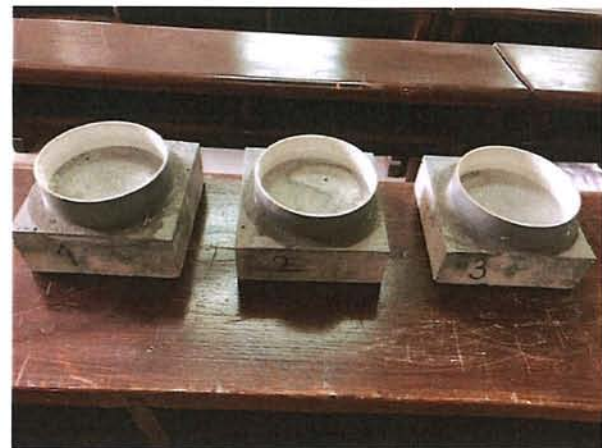
Figure 5.2. Samples after 25 cycles in the environmental chamber
