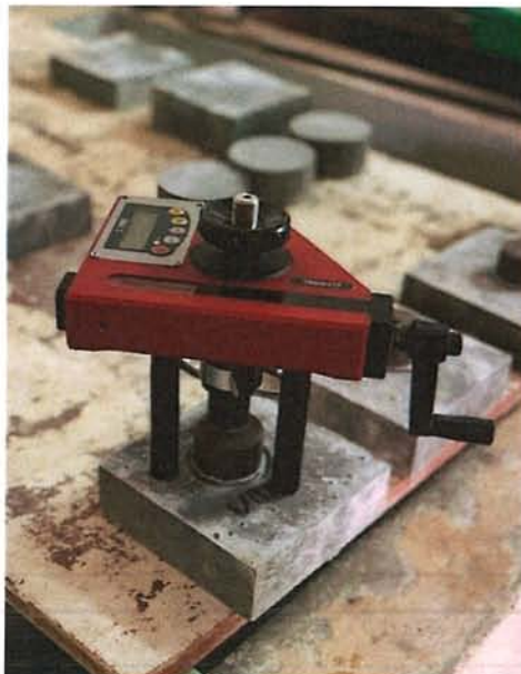
Figure 3.2. Equipment for „Pull off“ test
