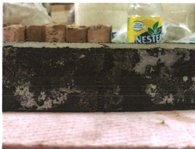
Figure 2.4. Appearance of samples with the addition of steel fibers after flexural strength test
