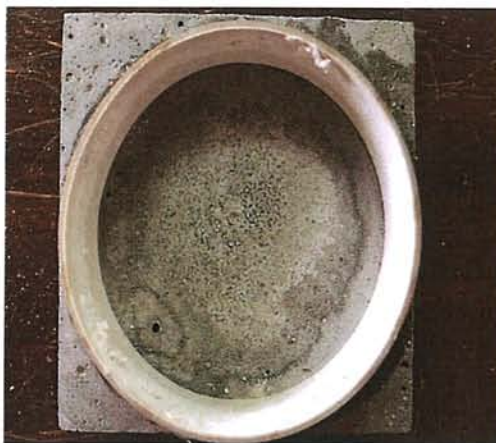
Figure 5.2. Samples after 25 cycles in the environmental chamber
