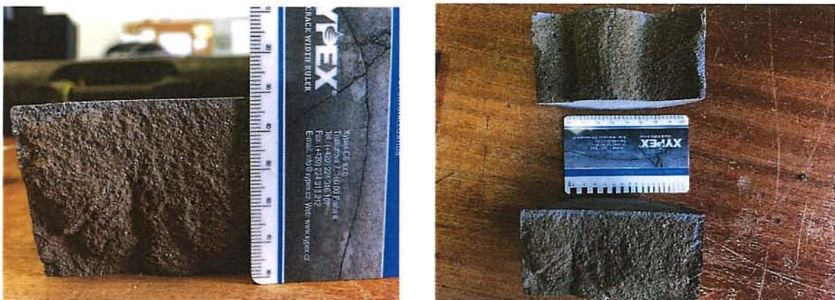
Figure 7.2. Appearance of the sample surface after treatment with silver nitrate solution
