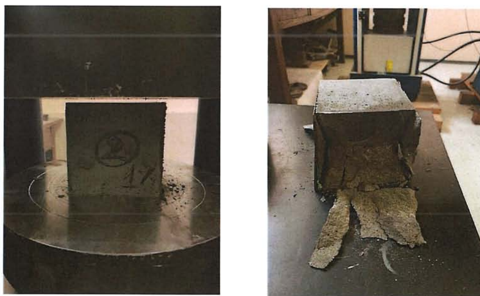
Figure 2.3. Prepared sample in equipment for compressive strength test and broken samples after test
