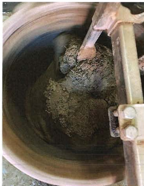
Figure 1.2. Mixture with fiber content during mixer operation and poured samples
