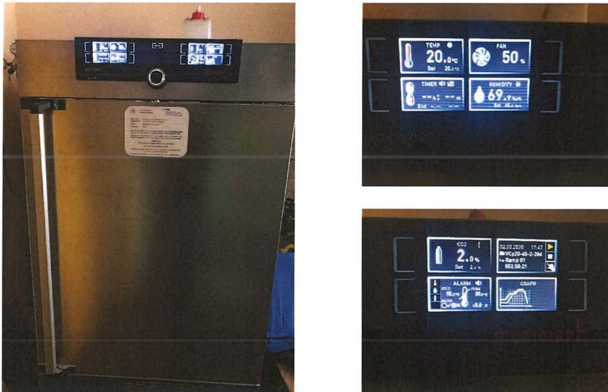
Figure 6.1. Environmental chamber for carbonation resistance test with set parameters ( CO_2 , temperature and humidity)
