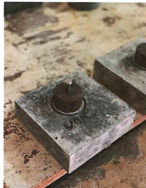
Figure 3.2. Equipment for „Pull off“ test
