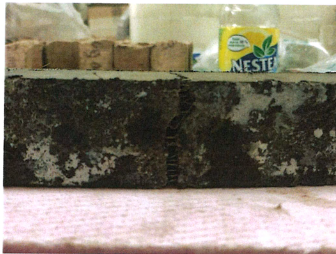
Figure 3.4. Appearance of samples with the addition of steel fibers after the flexural strength test
