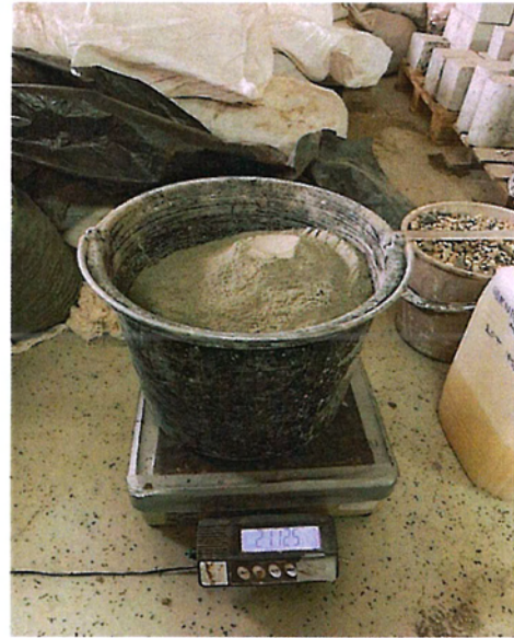
Figure 1.1. Preparation of components for making the mixture and precise weight measurement
