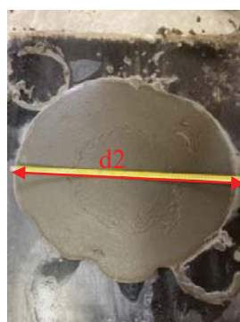
Fig. 1. Flow test-measuring the diameters
