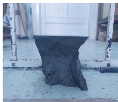
Fig. 2. Cube sample after compressive test
