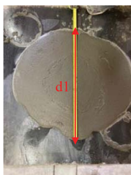
Fig. 1. Flow test-measuring the diameters
