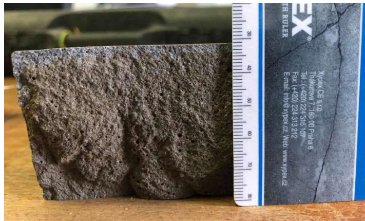
Figure 11. Appearance of the sample surface after treatment with silver nitrate solution
