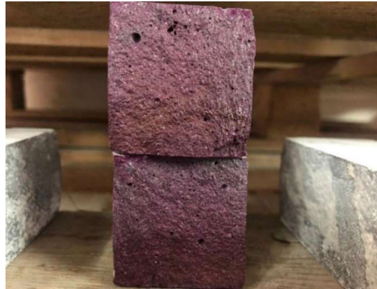
Figure 10. Appearance of the sample surface after treatment with phenolphthalein solution test
