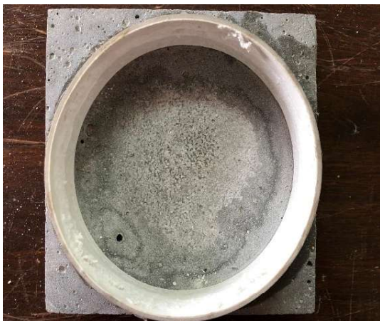
Figure 9. Surface of concrete sample after 25 cycles of freeze-thaw and salt attack
